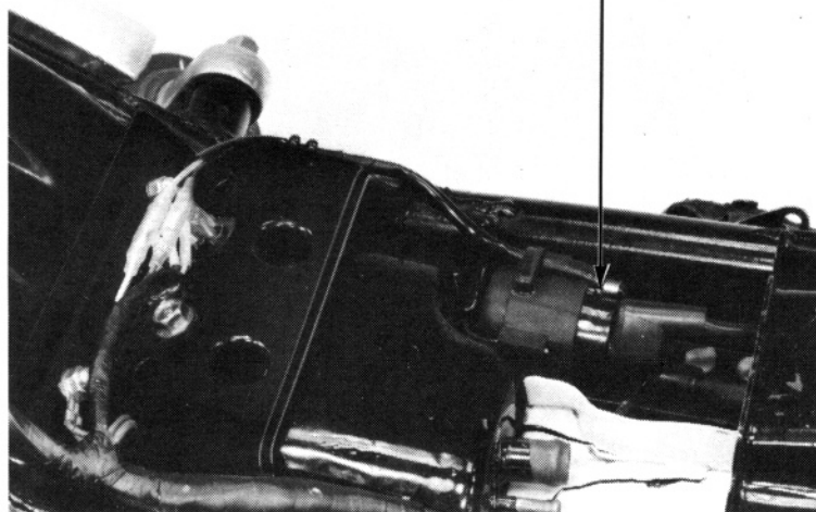
STARTER RELAY SWITCH
