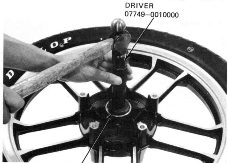
DRIVER 07749-0010000 ATTACHMENT, 42 x 47 mm 07746-0010300 PILOT, 15 mm 07746-0040300
