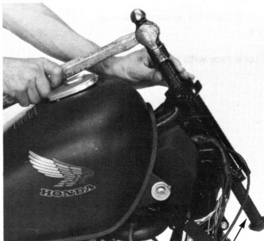
BEARING RACE REMOVER/INSTALLER 07946-3710400
