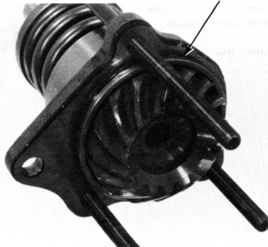
OUTPUT DRIVE SHAFT ADJUSTMENT SHIM
