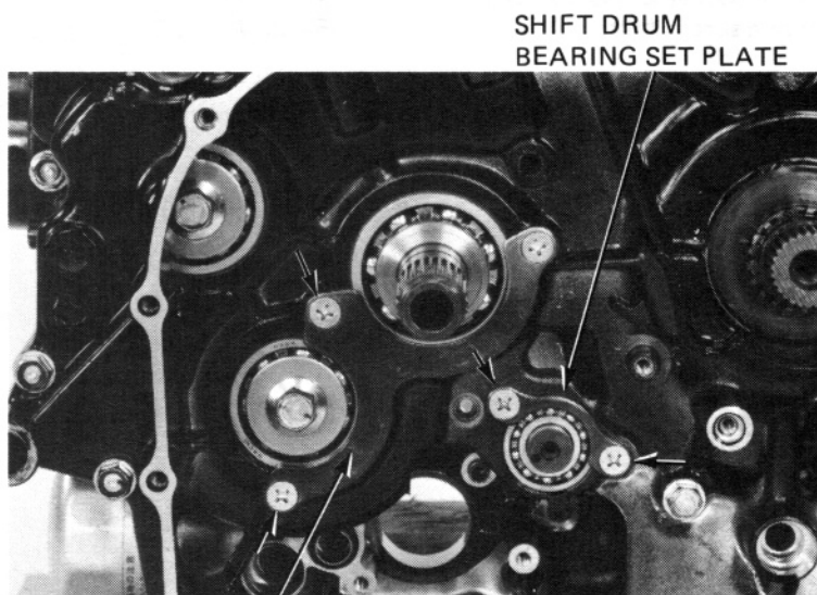
M & C SHAFT BEARING SET PLATE
